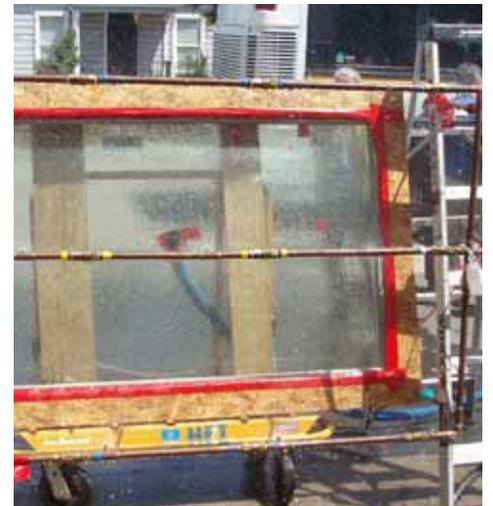
Wooden Window of Oakland hosted a tour through their facility and presented various possibilities on how to restore and maintain wood windows. Left: Removal of glazing from a freshly steamed window. Middle: CNC machine in action. Right: Pressure testing a wood window. Photos: Corri Jimenez.
